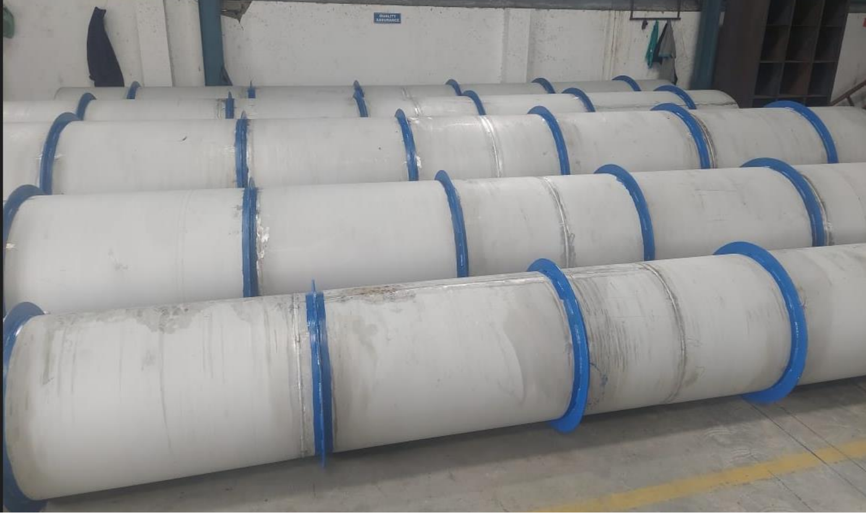
SS PIPES FABRICATION ( ROLLING & WELDING)
